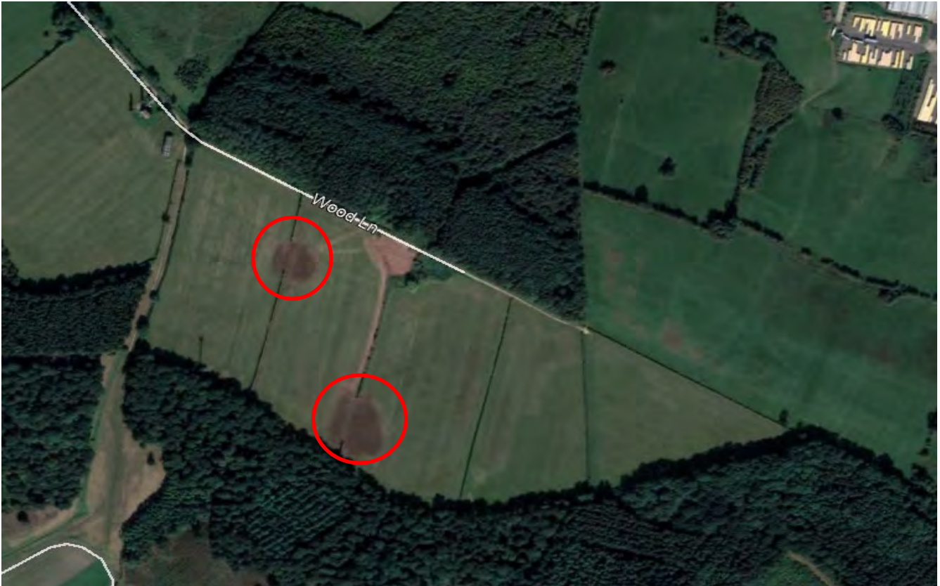
Areas of localised subsidence in Areas 1/8,9 and 1/10 2013
